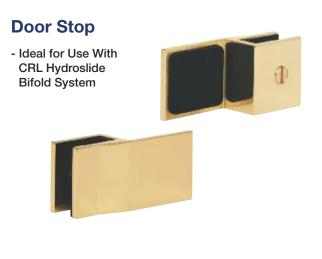
The Door Stop for CRL's Hydroslide Bifold Hinge System will protect the shower door from closing too far and damaging the door. The solid brass constructed Door Stop is dimensioned to accept 3/8" and 5/16" (10 and 8 mm) thick tempered glass when used in conjunction with our Hydroslide Bifold Hinges (HYDH037 and HYDH180). No glass fabrication is required.
