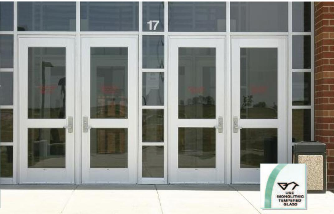
Durafront Doors and Frames are fabricated from tubular aluminum extrusions with a wall thickness of 3/16" (4.8 mm). These extra strong, long-lasting entrance packages are ideal for locations subjected to extremely high traffic flow. Durafront Entrance Packages are offered for center and offset hung doors. Offset hung doors are supplied with a pair and a half of heavy-duty hinges, pivot sets, or a continuous gear hinge. A variety of custom hardware is available upon request.
