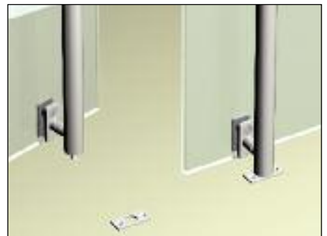
Glass Mount Detail at Latch at Floor With 777SP Flat Strike
