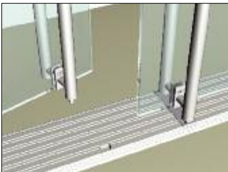
Glass Mount Detail at Latch With Threshold Prepped for Latch
