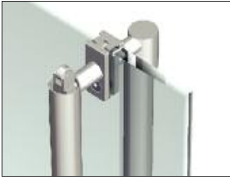
Glass Mount Detail at Latch
