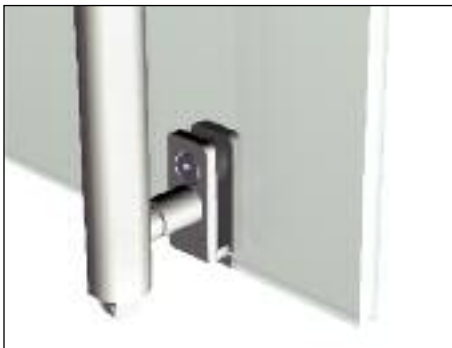
Glass Mount Detail at Latch
