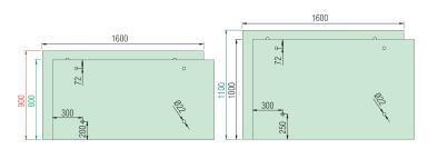
Glass: laminated safety glass consisting of heat strengthened glass with quadruple foil 8/1.52/8mm or 10/1.52/10mm
