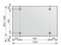
Glass: laminated safety glass consisting of heat strengthened glass with quadruple foil 6/1.52/6 mm or 8/1.52/8 mm
