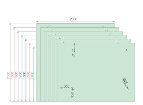
Glass: laminated safety glass consisting of heat strengthened glass with quadruple foil 10/1.52/10mm or 12/1.52/12mm
