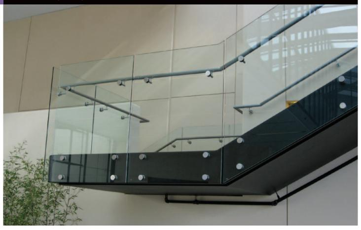
CRL's heavy-duty, point supported Glass Rail Standoff Fittings gives the installer more adjustment during installation for those tricky job site mounting conditions. The steel back plate can be fastened directly to steel, concrete, or wood substrates and shimmed as required with blocking.
