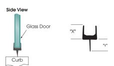
This ultra clear One-Piece Bottom Rail is snapped on the bottom of the door to achieve a seal. Because it is a single-piece sweep, it means the vinyl seal that hangs down from the sweep will firmly direct the water back into the shower enclosure.
