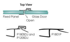
This Clear 180° Polycarbonate is snapped onto the fixed panel running inline with the door. P180SDJ and P120SDJ contain vinyl insert V600CSG. P1801P is all one piece.
