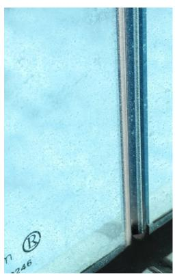
After the test, the glass panels were visually inspected and evaluated. The results showed that the panels remained unchanged in terms of their transparency. The PVB laminates showed edge clouds after 500 hours of testing. Due to the excellent edge stability of SentryGlas® interlayer, no undesired changes such as edge cloudiness, delamination caused by the humidity occur. Copies of the test report are available on request.
