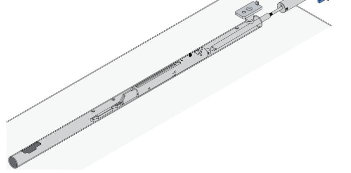
7. Unscrew and remove the Bolt from the Connection Rod .
