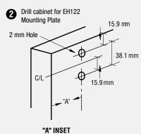
Overlay Hinge = 36.9 mm Inset Hinge = 36.9 mm Plus Glass Thickness
