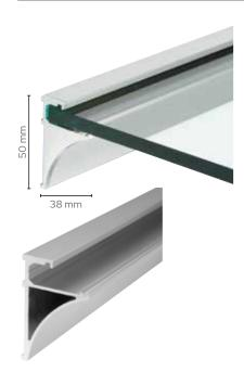
CRL Aluminium Shelf Extrusions are designed to support glass shelves without a lot of visible metal. The cleat easily attaches to studs with screws, and can support a shelf with a maximum projection of 305 mm. Offered in 2.4 m long Extrusions, you are no longer limited to "standard size" shelves. The Extrusions may be easily cut to size, and by installing matching End Caps the shelves make for a beautiful presentation.
