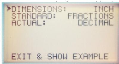
First, select the "DIMENSIONS" option by pressing the POWER button. Choose if you want your unit of measure to be millimeters or inches. Use the ARROW keys to toggle between units and press the POWER button to make your selection.
