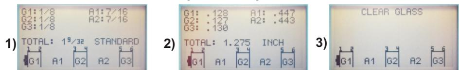
Display 1 shows fractional inches rounded to the nearest standard. Display 2 shows the actual measurements in decimal inches. Display 3 shows that the meter did not detect a low-E coating on G1 or G2. Since the GC3200 only detects coatings on the first 2 panes, you may be required to test both sides of a triple pane window to verify the presence of a low-E coating on the glass on the opposite side of the window.
