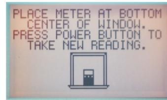
After the WELCOME SCREEN, the meter will go to its measurement reminder screen, reminding you to [place the GC3200 meter at the bottom center of the window for ALL MEASUREMENTS!!](#) This is the preferred measurement location that should be used for ALL MEASUREMENTS. Testing in this location will eliminate effects from glass that is flexing inward, resulting in a concave glass surface. The most accurate measurements of a window will be obtained in this location when using the GC32000 meter.
