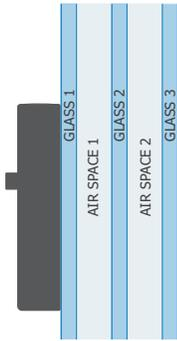
The GC3200 will display the thickness of each pane of glass, the thickness of each air space, and the total IG thickness. Depending on the thickness of the glass, the maximum allowable range for the total IG thickness changes according to the data below:
