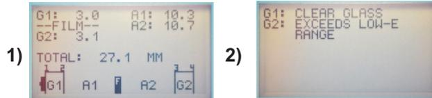
Display 1 shows the actual thickness of the window in MM. Since the “Standard” setting is set to OFF, STANDARD dimensions are not displayed. The word “FILM” indicates suspended film between the two panes of glass. Display 2 indicates that G1 does not have any low e coatings (“CLEAR” of any low-E coating). In Suspended Film Mode, the GC3200 will NOT test G2 for Low E Coatings.
