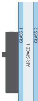
The GC3200 will display the thickness of each pane of glass, the thickness of each air space, and the total IG thickness. Depending on the thickness of the glass, the maximum thickness range for the total IG thickness changes according to the data below. **\*\*Note\*\*** these same dimensions apply when measuring a double pane window with suspended film.
