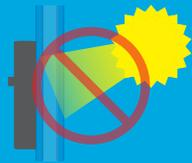
The Glass-Chek ELITE uses a laser to measure the thickness of the glass and air space. The unit may be affected by *extremely* bright lights or facing the sun directly. The screen will display this error message if this condition occurs. Simply move to a different location, go to the other side of the window, or shade the laser aperture. If the window is operable you may be able open the window and reach through the opening to block the incident light from the back side of the meter.
