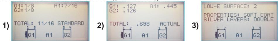
Display 1 shows fractional inches rounded to the nearest standard. Display 2 shows the actual measurements in decimal inches. Notice how the actual measurements in 2 are slightly different than the measurements in 1 because Display 1 shows the readings rounded to the nearest standard. Display 3 shows that the low-E coating is on surface 2, and it indicates that the coating properties are soft coat and have the performance of double-silver Low-E.
