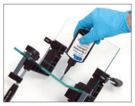
An important fact to always remember is that the smoother the bonding surface and the thinner the layer of adhesive, the stronger and more resilient the bond will be. A layer of too much adhesive reduces the strength of the bond, and increases the workload of removing excess adhesive.
