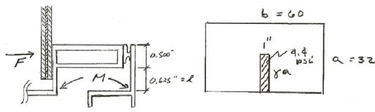
PERFORM BENDING AND SHEAR ANALYSIS PER UNIT LENGTH OF FRAME
